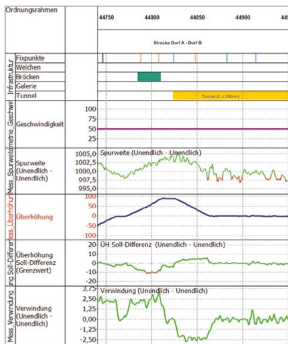
even produces its own measurement data. Alongside the classic track parameters of rail geometry and gauge, the height and distortion of the overhead contact wire is also measured. The next stage is to evaluate critical fault combinations. For example, exceeding the torsion limit combined with a gauge that is too narrow and a high line speed is much more serious than if the limit of the distortion occurs with an unremarkable gauge and low line speed.
