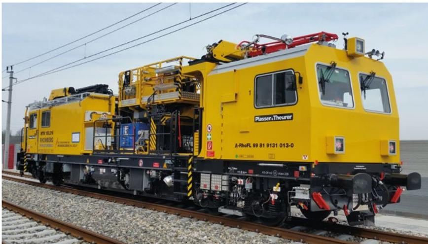
66 tonnes over 18 metres: the MTW 100 catenary maintenance vehicle.
