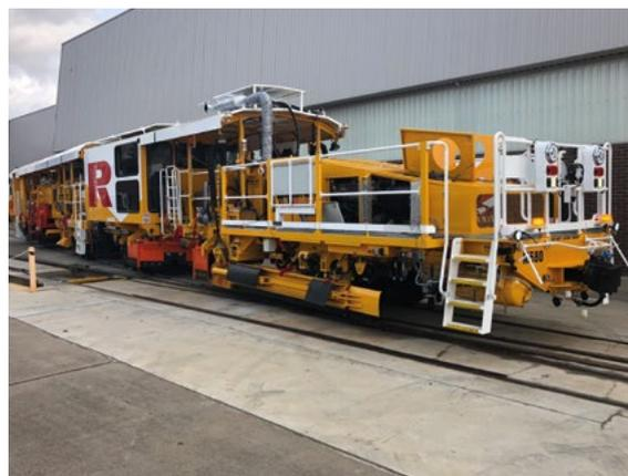
tests, high-speed travel at 110 km/h and parking brake tests on Sydney Trains' rail network's steepest slope. Now the SSP 303 as a resurfacing machine for points complements the M865 UNIMAT 08/275 3S tamping machine on the east coast of Australia.
