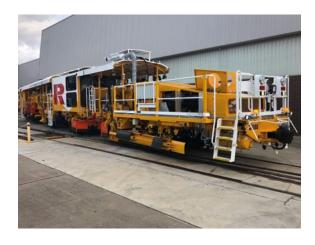
tests, high-speed travel at 110 km/h and parking brake tests on Sydney Trains' rail network's steepest slope. Now the SSP 303 as a resurfacing machine for points complements the M865 UNIMAT 08/275 3S tamping machine on the east coast of Australia.
