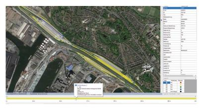
With MR.pro® our customer bremenports has a perfect overview of the railway infrastructure in the harbour of the Hanseatic city. The GIS viewer in MR.pro® displays all network database objects to scale. Every piece of information in the database can be mapped, parameterised and colour-coded: inventory and condition data, repair requirements, measures and projects.
